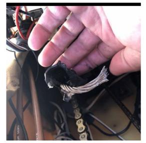
Afterwards worrying over how to get the steering fixed, the costs, effort etc., Evan took the steering/helm unit apart to trouble shoot the problem and found the assembly which held the cable to the chain had come apart, the shrink wrapping surrounding two heavy duty clips degraded, the clips wiggled loose and a circlip had fallen down into the auto helm mechanism, which caused the steering wheel to lock up (It was good we didn't try to force the steering wheel to turn)
